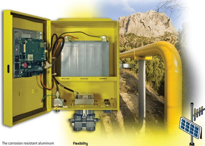
The corrosion resistant aluminum enclosure is rated Type 3RX and can be installed on a standard 2 "pipe. It can also be mounted on a wall, installed with optional Unistrut hardware or supported on the pipeline infrastructure by the sensor itself. For added flexibility, the pressure sensor can be mounted directly on the bottom of the enclosure or remotely, at a distance from the enclosure.
