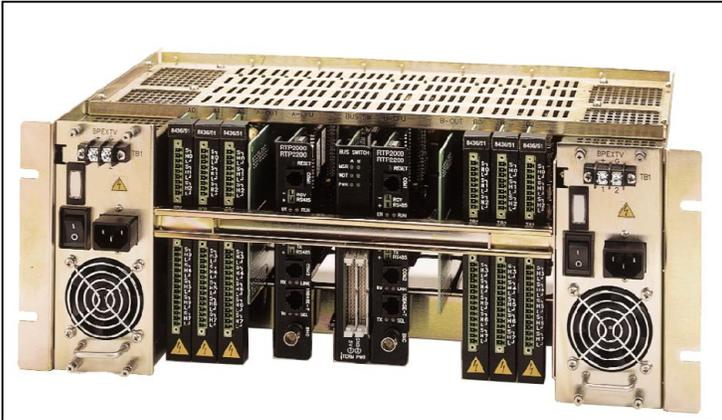
The basic RTP 2000 system includes a standard 19" rack-mountable chassis with an integral power supply, an embedded processor, and sixteen I/O option card slots—expandable up to a total of eight I/O chassis. The embedded processor, which includes 16MB memory, a high-performance Intel-base architecture, and an RTP bus controller, provides more than ample support to execute the most demanding industrial control strategy including cascaded and advanced feed-forward PID control.
