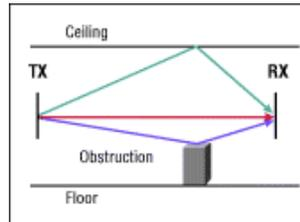
mode will continually switch between antennas, listening for a valid radio packet. After the beginning sync of a valid packet is heard, the radio will evaluate the sync signal of the packet on one antenna, then switch to the other antenna and evaluate. Then the radio will select the best antenna, and use only that antenna for the remaining portion of that packet.
